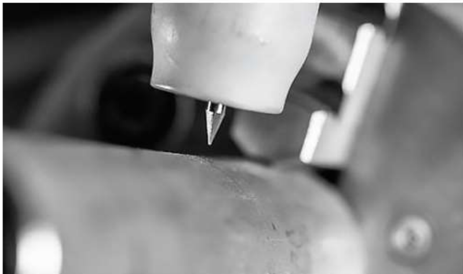
While tungsten electrodes are frequently used in welding, their structure, sharpening and alloy have a previously underestimated influence on consistently good product results in TIG welding. A reproducible weld seam is only possible if the electrode quality and geometry are outstanding.
